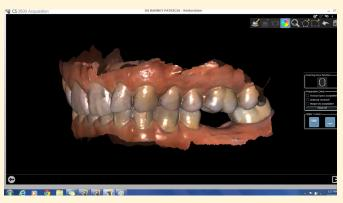
3Shape's Implant Studio software was used to plan a surgical guide and their Dental Design system was used to fabricate a customized gingival former.
