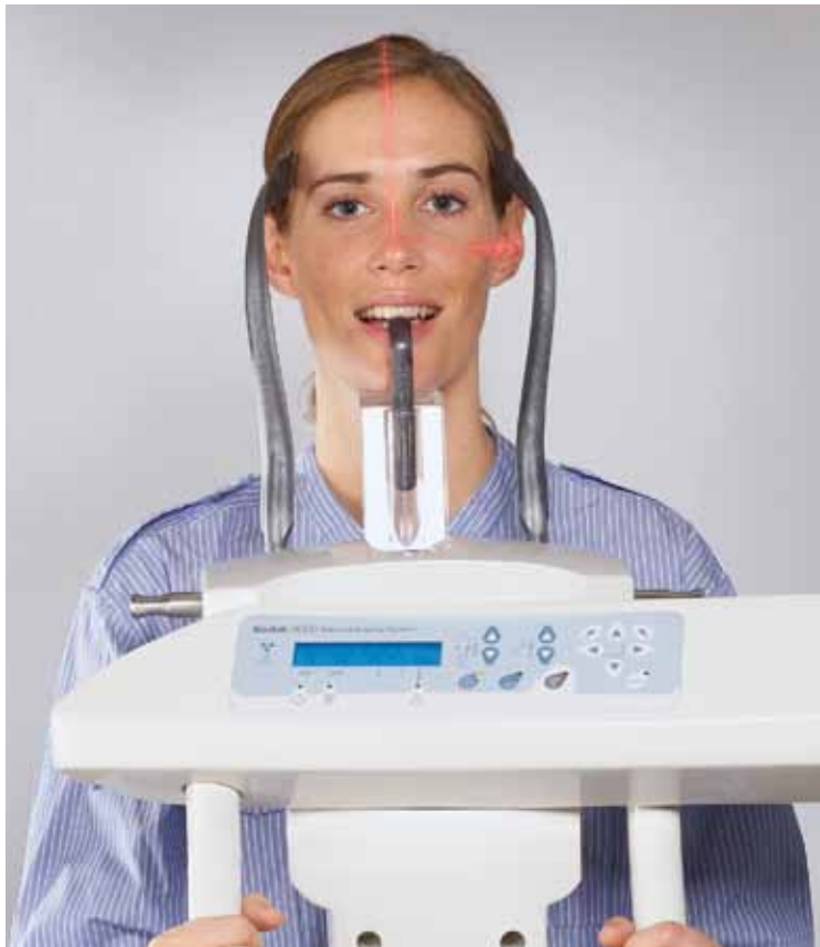
Figure 11 – Positioning guides; note the bite rod, head guides, and aiming light
